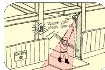
Alarm/warning speaker at constructions site
