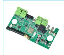
This Nemtek Connect Device Gateway 2G provides a connection from your Nemtek security energizer to the Nemtek Connect App. This App can remotely monitor and control these energizers and allows you to receive notifications and alerts.
