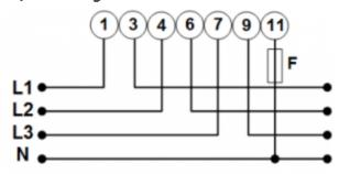
When used to measure a PV Inverter, terminals 1, 4 and 7 should face the PV inverter to ensure correct direction of current and power.
