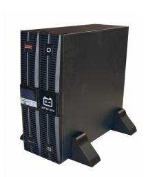
The UPS has a built in Static By-Pass feature which enables the machine to transfer the load to normal mains under certain emergency conditions, such as an overload. Once the condition causing the by-pass has been corrected the unit will automatically return to its normal operating mode.
