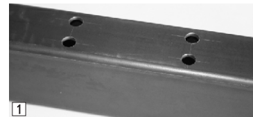
1 MARK OFF AND DRILL FOUR DIAMETER 10MM HOLES AS PER RECOMMENDED DRILLING PATTERN. SEE FIG 2A OR 2B
