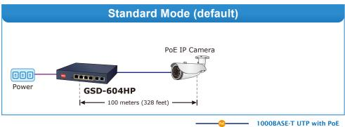
■ The VLAN operation mode features the port-based VLAN function that can help to prevent the IP camera's multicast or broadcast storm from influencing each other.
