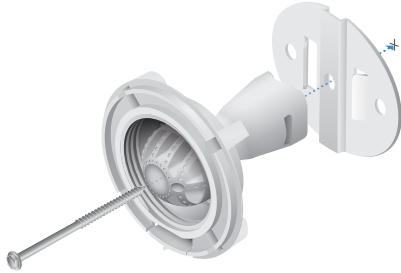
Installation Using the NanoBeam Wall Mount Kit
